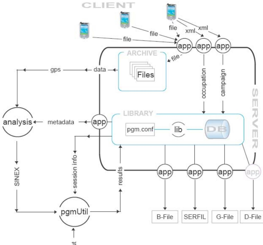
**Figure 1.** Schematic of the Pocket GPS Manager. It provides a modern geodatabase/web-based/distributed GIS environment for planning, collecting, analyzing, interpreting, and publishing GPS-based projects.
